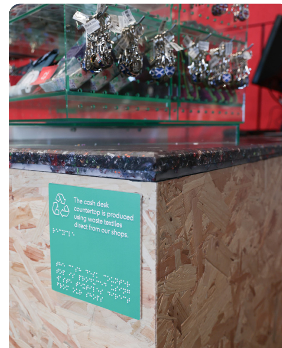
Shop countertop made from waste textiles
