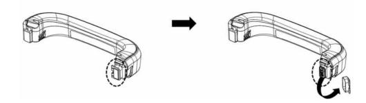
Figure 5. Removing the battery protection cap
