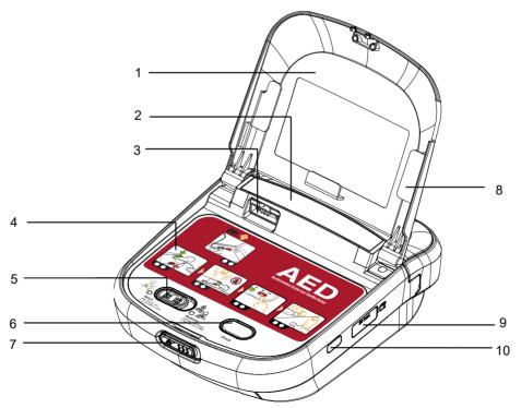
Figure 2. HeartOn A15-G4: Top and Right Panel Components
