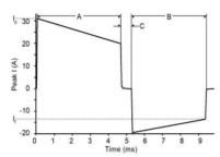
Waveform parameters are automatically adjusted as a function of patient defibrillation impedance. In the diagram at left, A is the width of pulse 1 and B is the width of pulse 2 of the waveform, C is the inter-pulse delay,  $I_p$  is the peak current, and  $I_f$  the final current.
